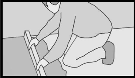
**Fig.57** - The curing/seasoning time of cement-based screeds is of essential importance. As far as conventional sand/cement screeds are concerned, this time is about 7/10 days per cm of thickness. If you are using premixed products, such as **Mapei's** Topcem Pronto or **Kerakoll's** Keracem Eco Pronto, follow the instructions of the manufacturer.
