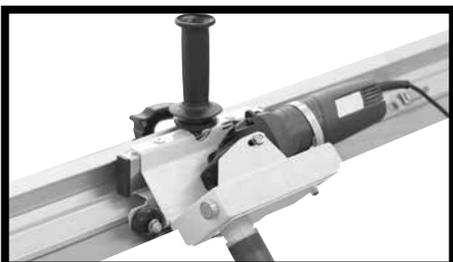
**Fig.14** - With tile cutter rulers, you can use hand-held angle grinders, fitted into special frames that can be "fit onto" the cutting guide. In this manner, you can provide both 90° and 45° cuts to obtain bevels and jolly pieces.
