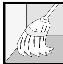
**Fig.36** - The support must be clean. Dust, oil, grease, dirt and debris must be removed as they may compromise adhesion of the adhesive.
