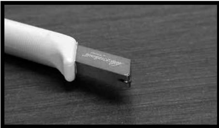
**Fig. 9** - You can obtain excellent results in terms of shape and clear cuts by engraving all versions of SLIMTECH with Silberschnitt 2000 special glass cutters made by **Bohle Italia** or with the manual tile cutter made by **Würth**. To achieve good cuts, never detach the glass cutter from the slab throughout the entire cutting operation.
