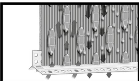
**Fig.56** - SLIMTECH 3plus and SLIMTECH 5plus can be installed directly on the CeraVent® Gutjahr® system. This system allows for wall installation (walls featuring salt and rising damp, damaged facades, mixed supports, prefabricated materials, etc.) and offers microventilation and uncoupling from the substrate.
