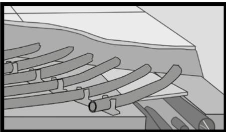
**Fig.59** - Before starting the heated floor system, wait at least 14 days after casting the screed. As prescribed by the UNI EN 1264-4 standard, in point 4.4, heating begins at an initial temperature ranging from 20°C to 25°C, which must be maintained for at least 3 days. Then set the maximum permissible design temperature and maintain it for at least 4 days. Once the floor has reached ambient temperature, tile installation can begin.
