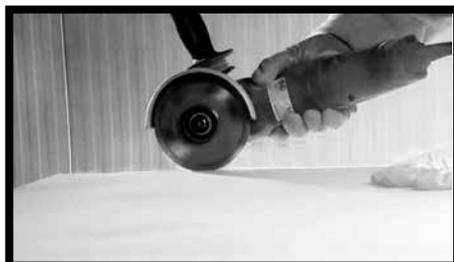
**Fig.21** - The same results can be obtained with sanding discs fitted onto hand-held angle grinders.
