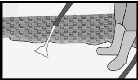
**Fig.58** - Follow the instructions of the manufacturer. Before installation, the screed must be sandpapered, dedusted and perfectly dry (the maximum permissible moisture content is 0,5%).
