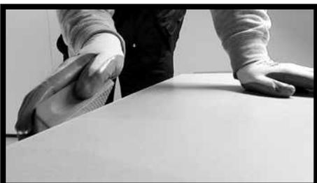
**Fig.20** - Edges can be finished by hand using abrasive diamond sponges or emery paper. With a light passage on the side of the slab, you can obtain a slightly rounded-off edge or with repeated passages a bevelled effect.
