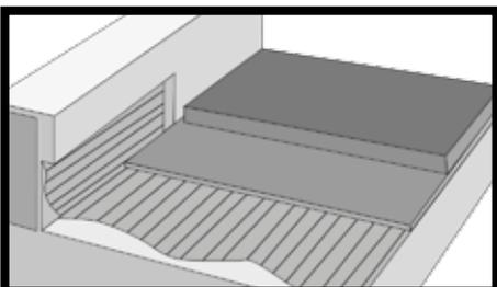
**Fig.60** - Concrete must be sufficiently cured (this takes about 6 months or even more, depending on its thickness, composition, thermo-hygrometric requirements, etc.) and must not feature surface treatments such as mould release agents, resin, anti-evaporation treatments, old adhesives, etc. Floor slabs must be insulated against rising damp.
