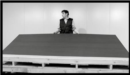
**Fig.1** - All types of 300x100 cm slabs of SLIMTECH can be lifted by one person only. Lift the slab with open hands. Slowly raise the longer side so as to eliminate the suction effect, due to contact with the underlying slab, and ensure a good grip.
