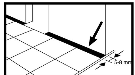
**Fig.71** - Around fixed elements of the supporting surface, such as walls, steps, columns, etc., it is **mandatory** to provide 5-8 mm peripheral joints.
