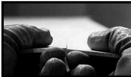
**Fig.11** - After engraving, it is sufficient to bend the slab to detach the two pieces.
