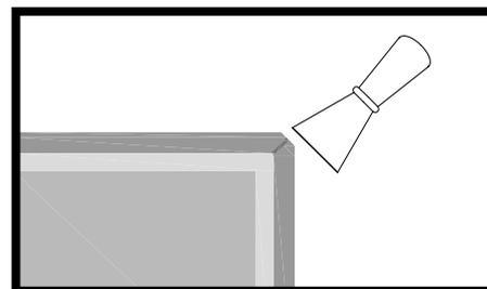
8 - Apply epoxy grout with a trowel (\*).
