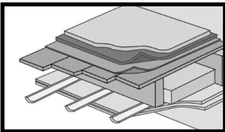
**Fig.53** - This construction system consists of a floor made of wooden planks secured by means of nails to a lattice of stringers. Installation of this construction system is similar to **installation on wood - Fig.38**: follow the instructions provided.
