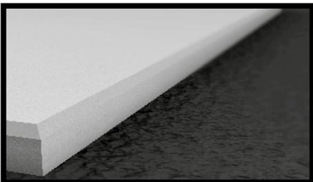
**Fig.30** - All versions of SLIMTECH can be bevelled. To obtain curved edges, use a numeric control machine with a 5-axis disc. Different discs are available for obtaining a variety of edge finishes. Operating speed must be tested beforehand.
