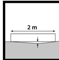
**Fig.34** - Flatness checking is performed using a levelling rod with a length of at least 2 metres. Place the rod on the slab in all directions. The permissible tolerance is 2 mm.
